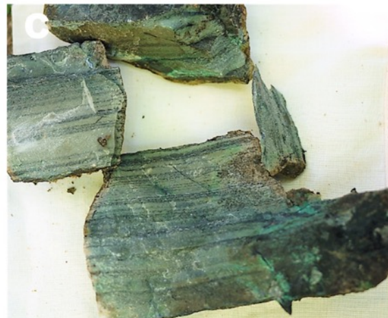
C) Upper Jurassic Sarayaquillo Formation, laminated siltstone to shale with chalcocite replacing pyrite and organic material. Typically contains 2-6% Cu and 15-60 g/t Ag and averages 0.5-5 metres thickness when exposed within 110km strike
