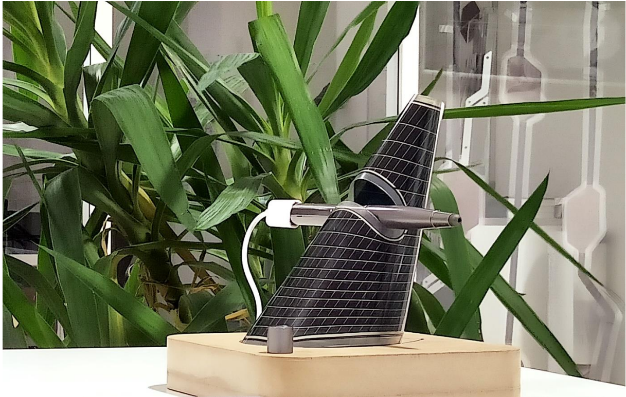
Solar driven power bank charger made by free-form OPV in a 3D configuration
