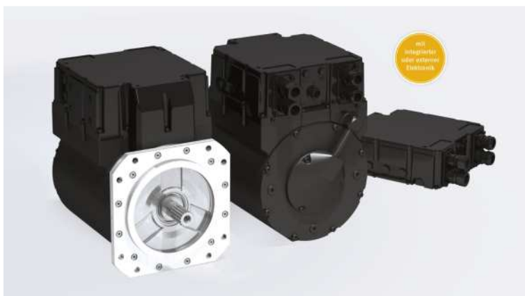
Fig. 2: The drive concept powerMELA® consists of a combination of permanent magnet synchronous motor and power inverter for the four-quadrant operation and is suitable as a hybrid or purely electric drive system for commercial vehicles and mobile working machines
