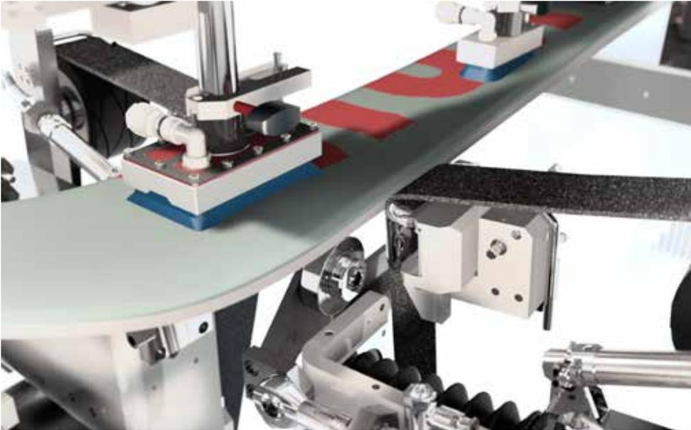
The best from belt and disc grinding. The unique process grinds all functional areas of the ski from shovel to tail to RACE EDGE quality. This results in the maximum durability of the sharpness combined with a removal which is gentle on the material.
