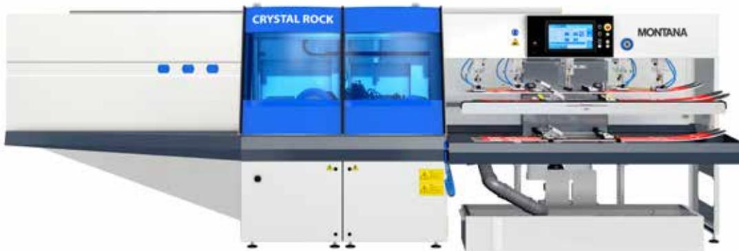
The wide grinding stone makes the CRYSTAL ROCK the optimal system for small and medium-sized shops. Also ideal as it can be used for both skis and snowboards.
