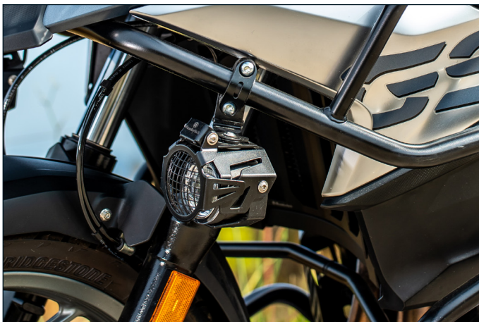
The lamp protection grille consists of a robust, black coated metal structure
