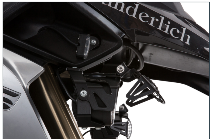
The headlight and grille are easy to clean thanks to a practical folding function
