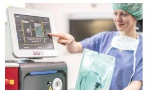
The automatic laser fiber recognition using an RFID antenna provides the user with very convenient and efficient identification of the laser-fiber size. Recognition can also be carried out in the packed sterile status of laser fibers. A flexible ureterorenoscopic lithotripsy with the COBRA vision and the new MegaPulse 70+ Laser from Richard Wolf was also presented at the EAU Congress in a pre-recorded video carried out by Dr. Michael Straub,
