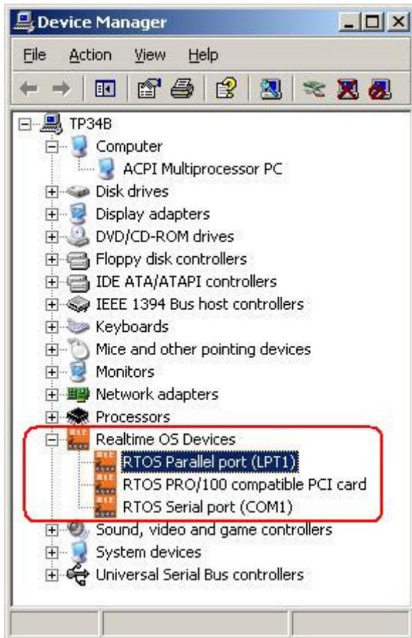
Within the RTOS there are two methods for detecting whether a device can be accessed or not. For PCI devices usually the PCI vendor and device ID can be used. For other devices (as well as for PCI devices) the device name (e.g. RTOS PRO/100 PCI card) can be used.
