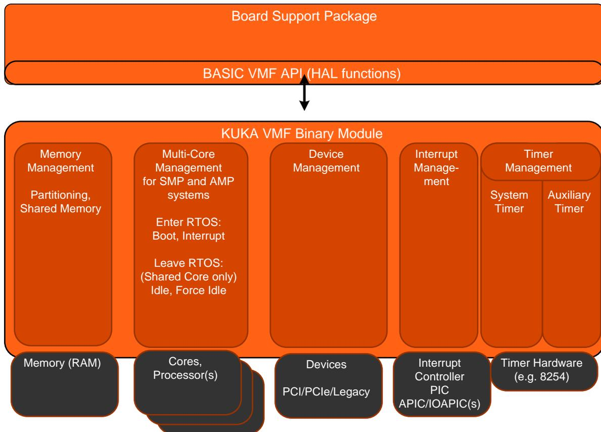
When porting system software (e.g. a RTOS Board Support Package) to run with the KUKA RTOS-VM there is no need to directly access PC hardware like timers or interrupt controllers.
