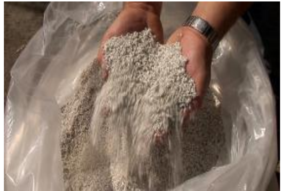
Fig. 2: The end product: agglomerate with high bulk density and excellent flow properties
