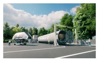
"Hyperloop" is the umbrella term for innovative high-speed transportation systems moving passengers and goods over long distances. The concept envisages electrically powered transport pods, propelled at travel speeds of over 800 km/h within sealed vacuum tubes. The TUM Hyperloop research project was established in the wake of
