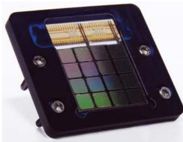
*Actual Dimensions: 27mm x 30mm - The SPMPlus is the first solid state alternative to the analog Large Area Photomultiplier Tube*
