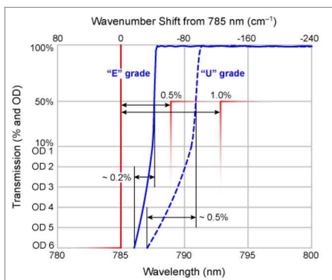
*RazorEdge filters are specified with a guaranteed “Transition Width,” or maximum allowed spectral width between the laser line, at which blocking is guaranteed to be OD > 6, and the 50% transmission point.*
