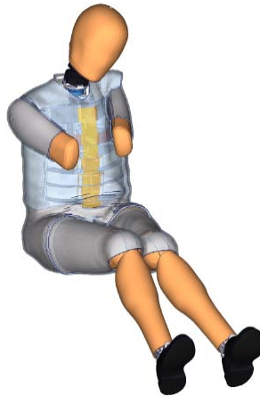
World SID 50 th dummy deformation mode under loading in a barrier test
