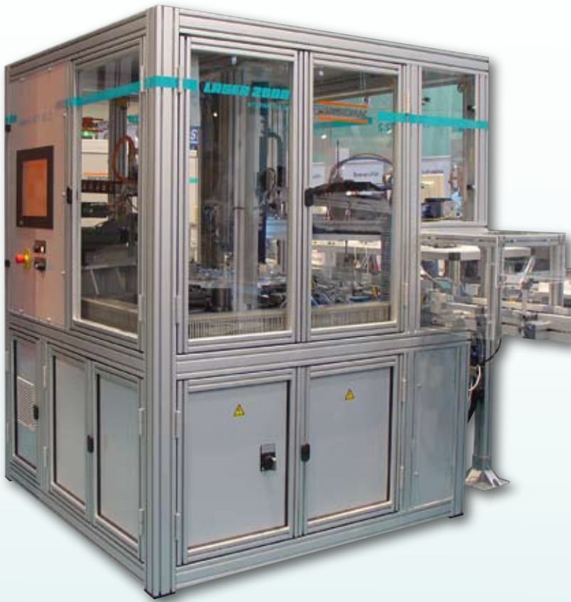
MC-Jet V2.2 with indexing table for full automatic operation
