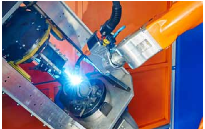
Photo 2: CLOOS has developed the fixture specifically for Halder.
