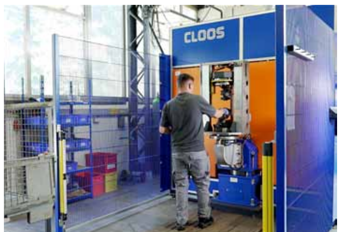
Photo 3: The two-station design allows for simultaneous welding and loading of the compact cell.
