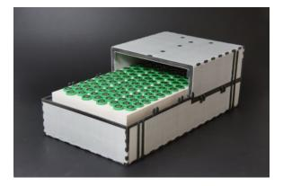
Battery module housing consisting of a thermally insulating polymer foam (black) covered with continuous fibre reinforced (CFRTP) facesheets, manufactured using a hybrid in-situ process in only 2 minutes. Photo: Fraunhofer LBF
