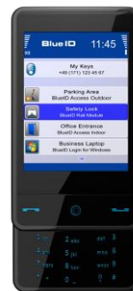
Image 4: The mobile phone becomes the bunch of keys: BlueID Rail Module grants access. Permissions are transmitted with RSA/AES encryption
