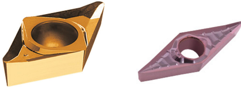
Picture nos. 10-05a AO_EB-WSP-Alu + 10-05b AO_EB-WSP-ASF High-positive indexable inserts from market leader ARNO Werkzeuge achieve top finish quality by optimising chip evacuation due to their ground circumference and polished surfaces.
