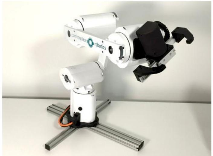
Mover5, 5-achsiger low-cost Roboterarm inkl. Parallelgreifer.
