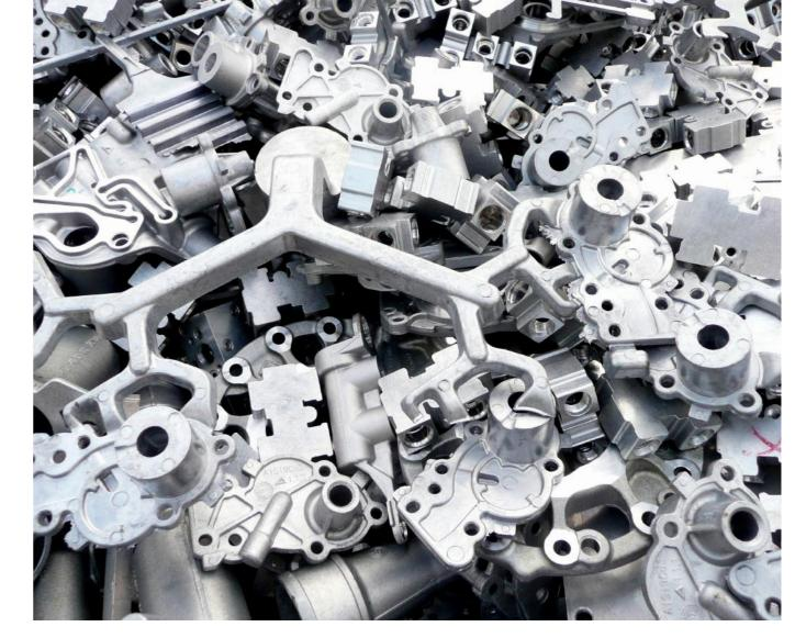
For the most efficient use of raw materials in the production process, the processing of reject materials and by-products of the foundry and machining industries is increasingly gaining in importance.
