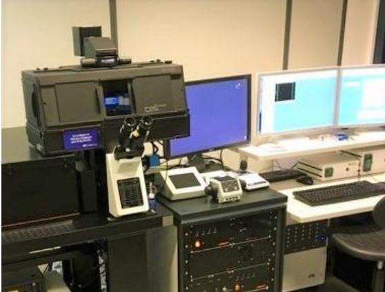
STED-AFM system incorporating JPK NanoWizard® - the Lafont Group
