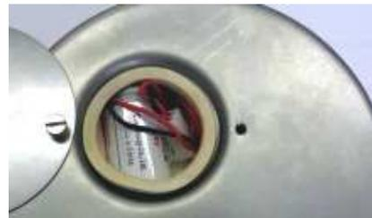
For replacing the battery just loosen a screw at my backside and ease the other one, pull out my heart at the cable. Lay it in, a little bit set off and close me again.
