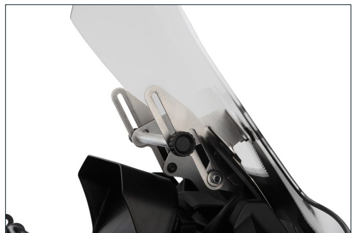
Well thought-out mechanism with slide guides guarantees that you can find your personal setting
