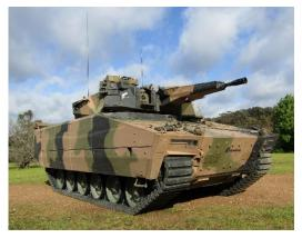
With the flexibility of the CRT fitted to the Lynx, the platform can be configured for a lighter all up weight (due to weight saving in track) to allow easier air transportation and to potentially reduce overall running costs through the service life of the vehicles.
