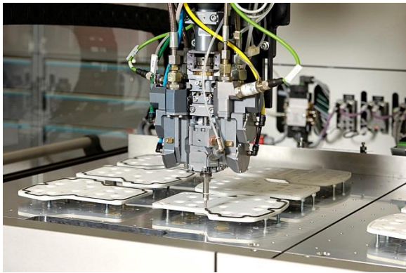
2-Component Formed In-Place Foam Gasketing with Fermapor® K31 polyurethane foam sealing
