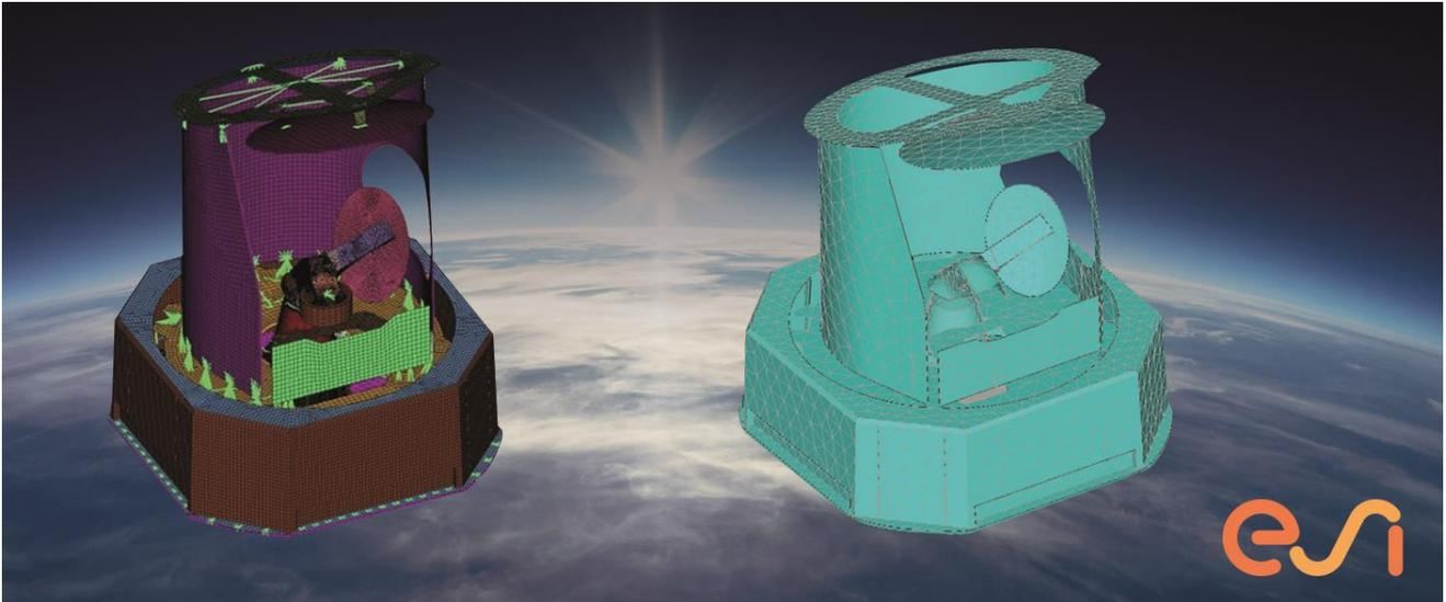
Image : FEM and BEM vibro-acoustic simulation models of a satellite payload for space applications with ESI VA One.
