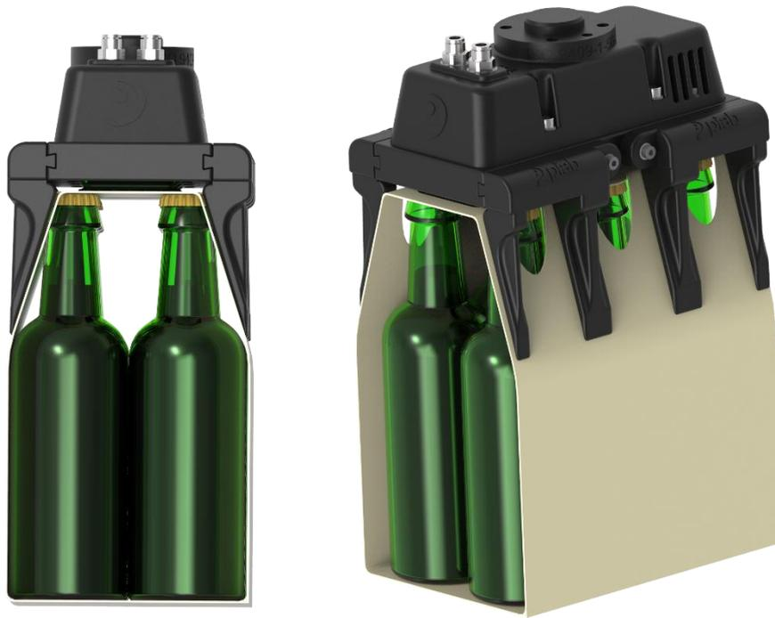
The gripper gently but firmly holds and lifts the sixpack without any damage to neither bottles, nor carton, nor label.
