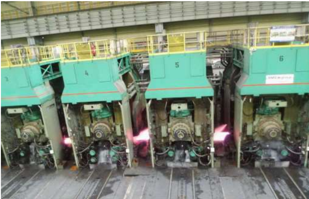
Finishing mill stands F3 to F6 during hot strip rolling.
