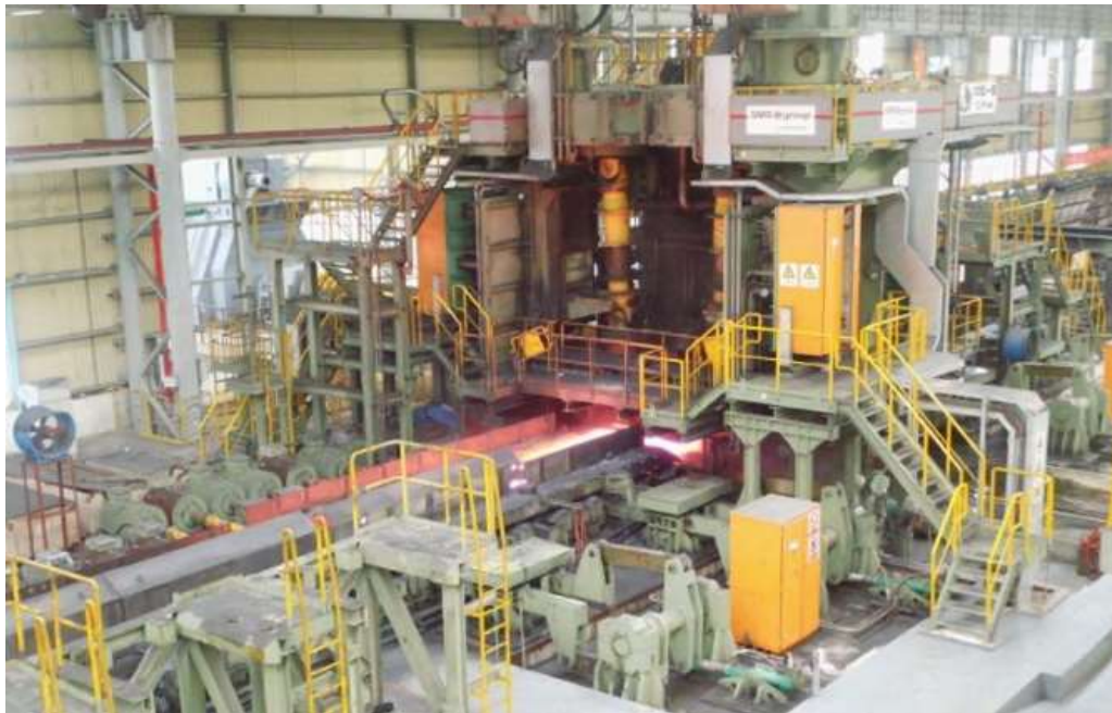
Roughing mill stand R2 with edger.
