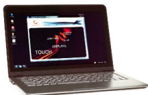
Figure 7. A 13.3” CNB touch sensor integrated in an Intel Ultrabook reference design (left). Reflections from the touch display with CNB and ITO touch modules (right). There is an air gap between the display and the touch module.
