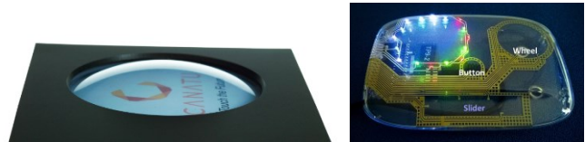
Figure 8. A 5” dome shaped CNB projected capacitive multi-touch sensor (left). A 3D shaped CNB FIM demonstrator with touch (right).
