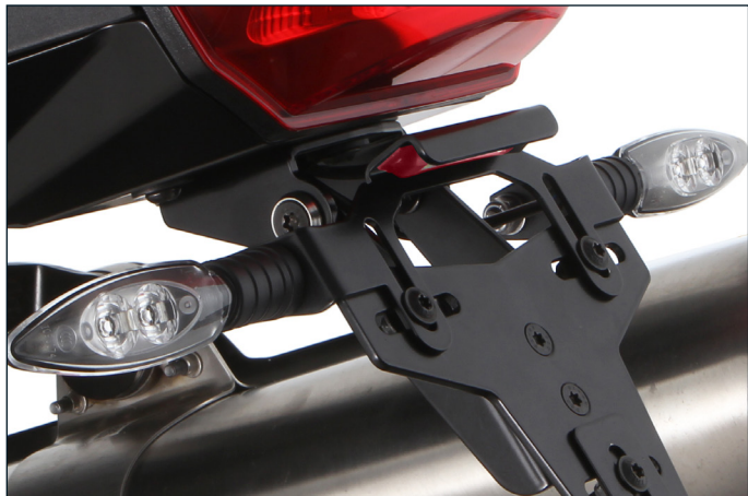
The licence plate holder comes with discreet LED licence plate lighting ...
