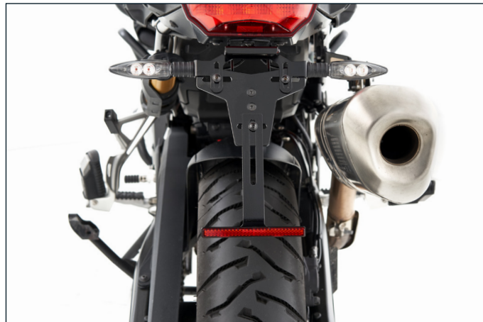
... and incorporates an inconspicuous, slim but widely designed reflector
