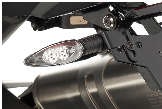
The original indicators can be combined with the conversion. Alternatively, Wunderlich offers the M-Pin indicator set with matching indicator bracket (Item-No.: 38983-002)
