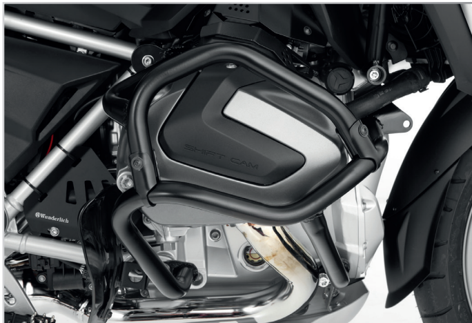
Protects the new ShiftCam cylinder head particularly effectively: Wunderlich engine guard with extension
