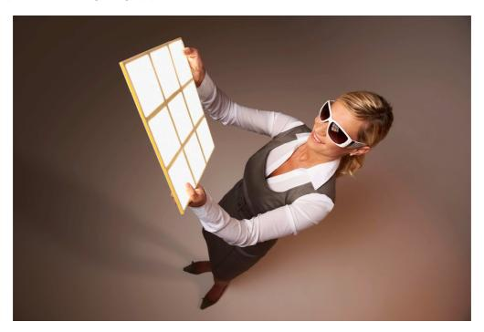
The Organic Light Emitting Diode (OLED) technology is the first real area light source technology in history. OLED lighting elements allow complete new lighting integration opportunities in different applications. Due to the slim form factor, it is possible to realize lighting solutions with very thin elements and high lighting homogeneity.
