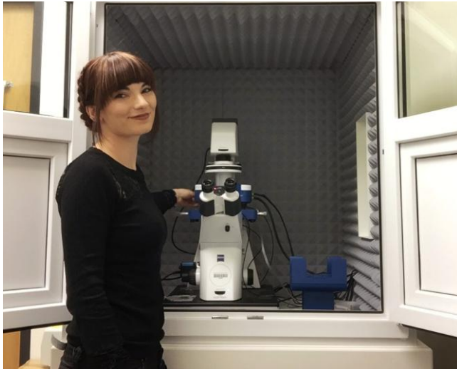
PhD student, Ilaria Pecorari, of the Mestroni Lab with the JPK NanoWizard® 4a AFM measuring mechanical behaviour of single cells.
