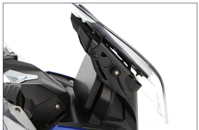
Ergonomically located knurled wheel for easy adjustment, even on the go
