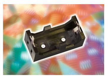
The BX0123 is designed for single CR123A cell accommodation with base or PCB mounting. Two fixing holes are provided for base mounting and PC spills for PCB mounting.
