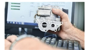
H 2 recirculation blower
