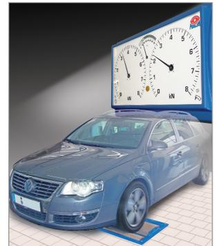
MAHA Roller brake tester MBT 2100 with large, easy-to-read analogue displays for measurement values
