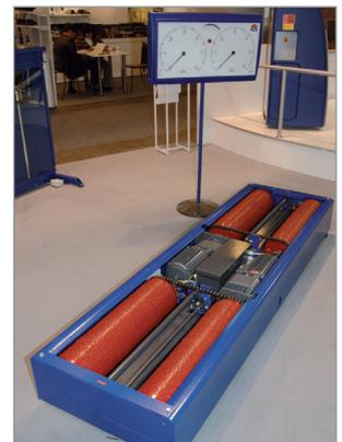
Complete unit of the MAHA Roller Brake Tester MBT 2100. Here with analogue display on pedestal
