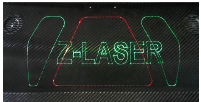
Pic1: ZLP's laser projection on composite material/carbon
