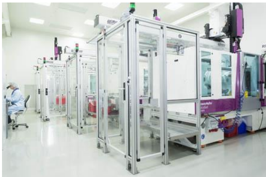
Image ref. 43-03 TB_SC-Reinraum.jpg. The Trelleborg Sealing Solutions facility in Stein am Rhein is equipped with class 100,000 (ISO 8) and class 10,000 (ISO 7) cleanrooms. The most recent round of expansion doubled site capacity.
