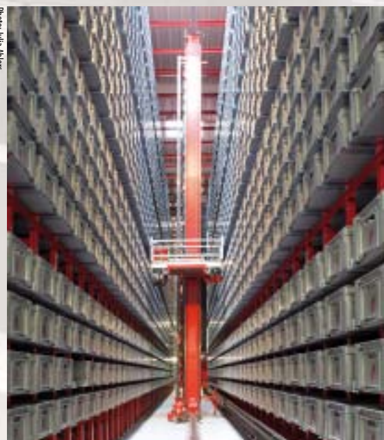
THE AUTOMATED SMALL PARTS WAREHOUSE (AKL) houses 24,000 containers, which are stocked completely automatically.
