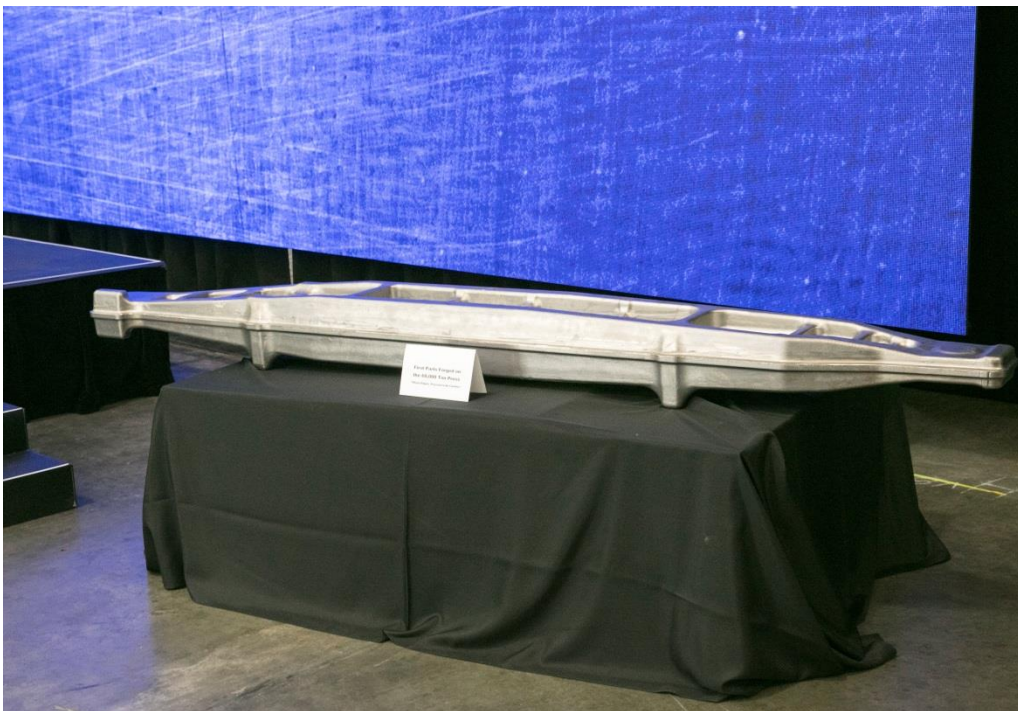
One of the first parts forged on the 60k press.
