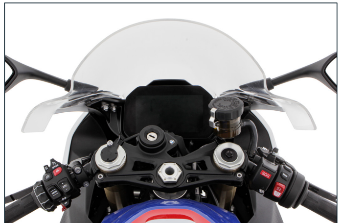
5 mm windshield thickness ensures mechanical and aerodynamic stability
