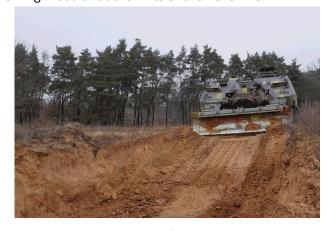
few minutes, it can cut a 160-metre-long and nine-metre-wide path through minefields and obstacles. When used together, the two Plofadder systems alone can clear a minefield up to 250 metres deep. The integrated lane marking system shows follow-on forces the cleared lanes, even in poor visibility or at night.
