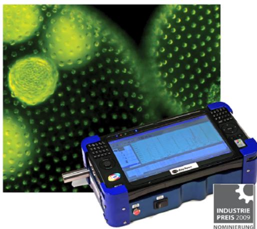
Unique 1064nm Raman Spectrometer resolves fluorescence issues seen at lower wavelengths : While algal oil is similar to other vegetable oils in terms of fatty acid composition, the oil productivity of microalgae, on an annual per-acre basis, could potentially provide 100 times greater yield than soy and 10 times greater yield than oil palm. Utilizing BaySpec's unique Nunavut 1064nm designed system, researchers were able to overcome issued with fluorescence seen at lower wavelengths.
