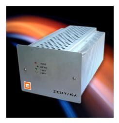
All models include remote sensing, Over-voltage/ Over-current/Over-temperature protection, LED indicators for DC-OK or Fail conditions and isolated fault signalization as standard. Further these power supplies can be used individually or up to 3 units can be connected in parallel for high power or N+1redundant power systems by incorporating built-in ORing Diodes/FETs.
