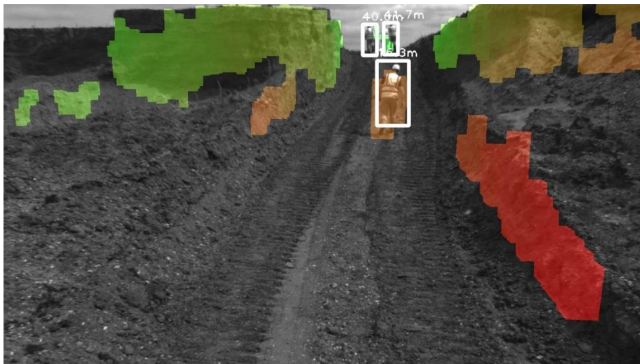
3D terrain mapping by ITK Engineering detects people and objects in rough terrain and alerts the driver to potential hazards. © ITK Engineering
