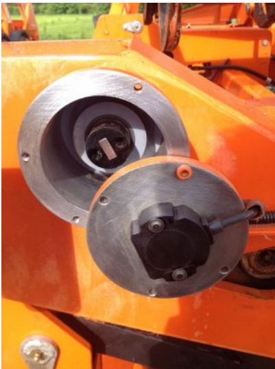
Image: RFC-4800 application example – steering feedback measurement on agricultural machinery
