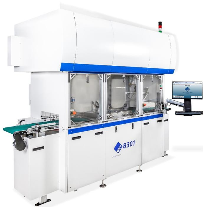
*The SST 8301 Automated Vacuum Soldering System placed at Fraunhofer IISB.
