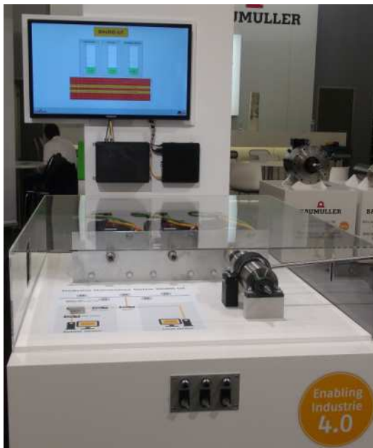
Fig. 3: BAUDIS IoT is an IoT-capable diagnostic and communication system that allows for a simple networking of machines and systems via the Internet and the intelligent analysis of data. Smart data analysis is used to avoid production errors and to increase productivity, all automatically through a self-regulating machine learning process
