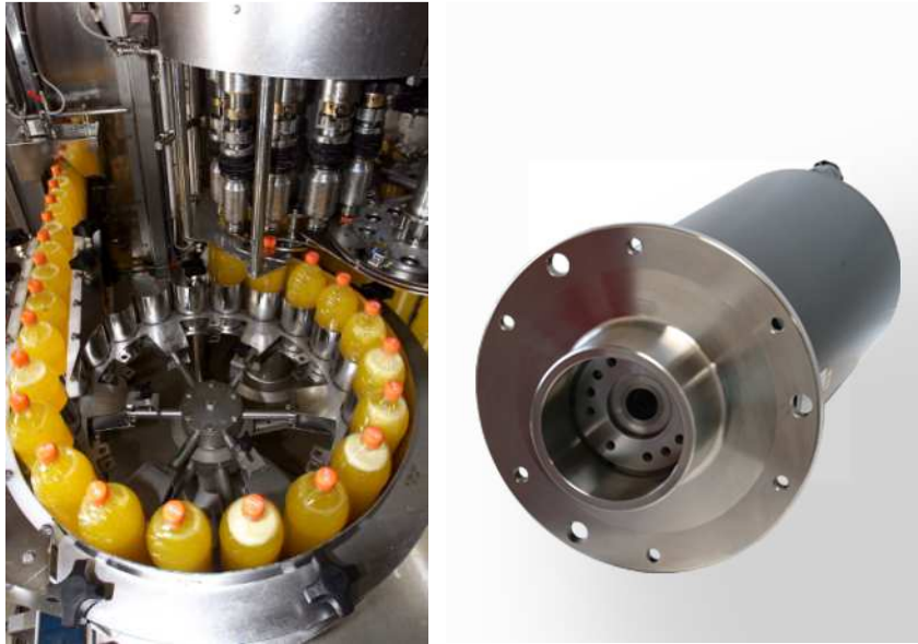
Fig. 2: The extremely compact high-torque motor DST2 80 (right), which among other things is used as a drive of starwheel columns for container transport in filling machines (left) in the beverage industry. The direct drive is thermally tightly encapsulated in a stainless steel pipe and impresses with very low self-heating and easy cleaning | Image left: Kronos
