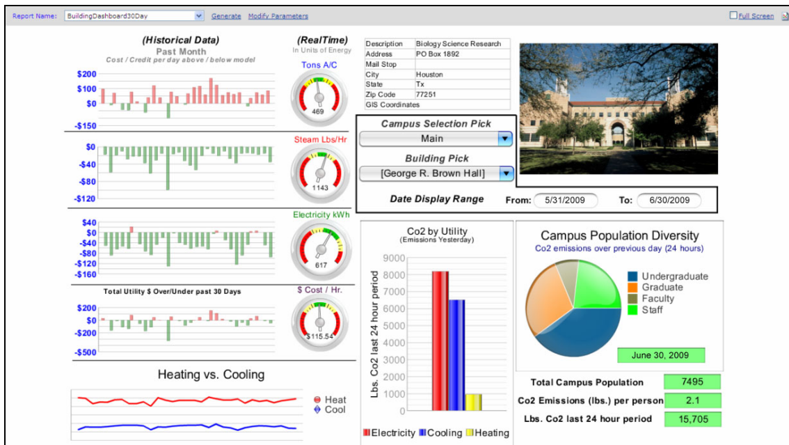
Figure 5. A graphical building dashboard displaying energy consumption and emissions information.
