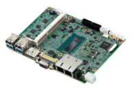
Advantech has developed an optimized thermal solution for MIO-5271, making fanless design possible on this kind of compact, high performance platform. MIO-5271 also has both iManager and <u>SUSIAccess</u>, developed by Advantech, integrated to monitor and control system operation remotely and effectively. These tools increase system reliability and provide a smarter software framework for the embedded customer, helping to speed up time-to-value for IoT & intelligent system design.
